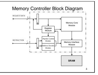
REQUEST DATA is a bi-directional I/O bus that is used for 72-bit reads and writes to the memory. The MC returns Programmed I/O (PIO) read data to the host environment on this bus. It also provides a CPU interface to read/write of the MC's internal registers, and the SRAM. The commands are provided to the MC on the INSTRUCTION bus to perform reads and writes.
