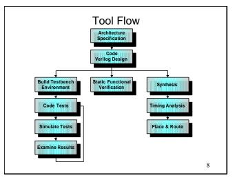
The tool suite used was Solidify from HDAC, Inc. for static functional verification and Synopsys Design Compiler for synthesis of the design. Other tools used were VCS and Virsim from Synopsys for simulation and Specman from Verisity for testbench development.
